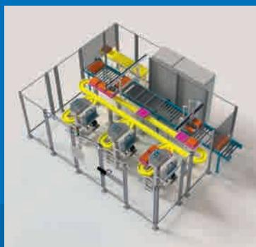
*Fully automated and customised end-of-line leak tests for battery cells.*
